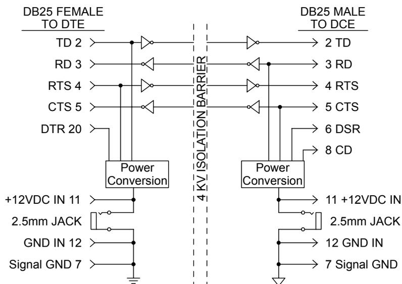
When connecting the isolator it is recommended that all device output signals be connected. The unit derives power from these signals, even if they are not used by your system. On a DTE device, with a DB-25 pin connector, the following lines are outputs:
