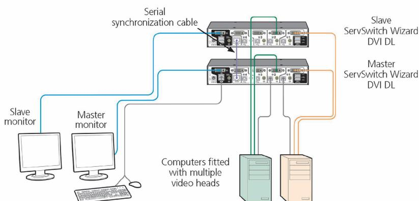
FIGURE 3-17. SYNCHRONIZING MULTIPLE UNITS
