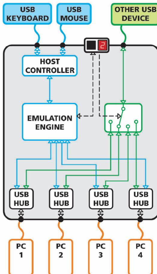
FIGURE A-1. EMULATED AND ENUMERATED SWITCHING
