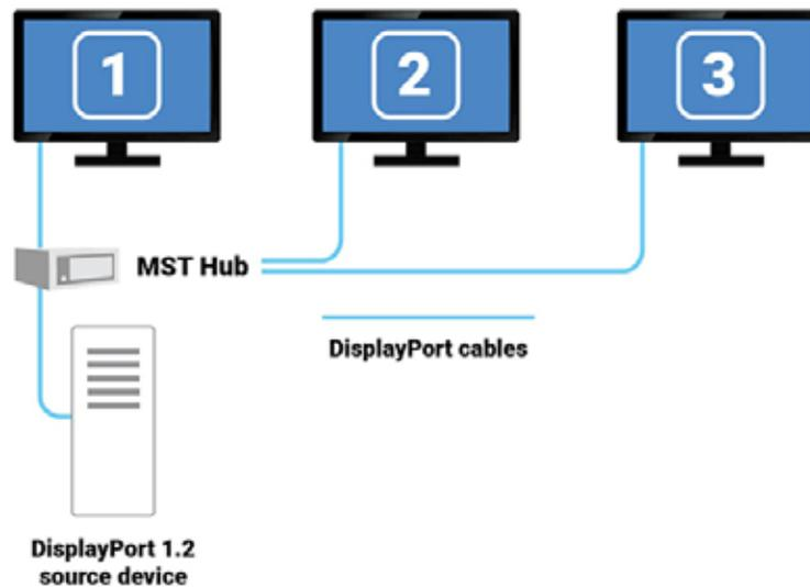
In the two examples above, 3 monitor connections are shown. But MST supports up to 5 monitors at 1680 x 1050 (WSXGA) resolution, 4 monitors at 1920 x 1080 (1080p) or 1920 x 1200, 2 monitors at 2560 x 1600 (WQXGA), or 1 monitor at 3840 x 2160 (UltraHD, 4K) or 4096 x 2160 (4K x 2K).
