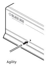
Use a straightened out paper clip to press the reset button while powering on the unit
