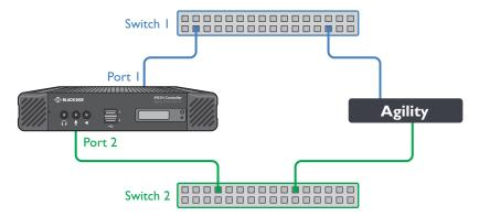
The 'Separate Device Networks' option mentioned earlier would be enabled on the iPATH Agility Controller and the respective network connections on the endpoints are connected accordingly (e.g. copper to copper on only switch 1 and SFP to SFP only on switch 2).
