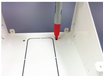
Figure 2-6. Transfer the hole location to the desktop.
