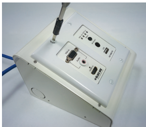
Figure 3-3. Secure the faceplate to the device.
