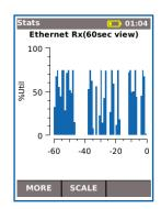
Real time display of broadcast network traffic shown as a percentage of port speed for the previous 10 minutes.
