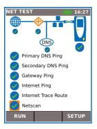
View network illustration to verify test results of each network component.
