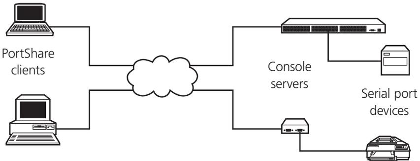
PortShare is supplied free with each console server, and you are licensed to install it on one or more computers for accessing any serial device connected to a console server port. This Quick Start walks you through basic configuration. For more details, refer to the PortShare chapter in the user's manual on the CD-ROM.
