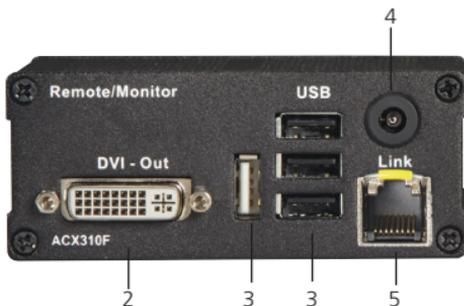
Figure 2-4. ACX310 receiver's back panel.
