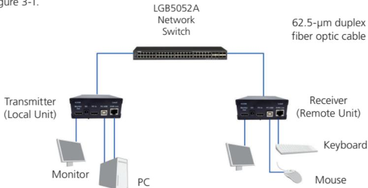
Figure 3-1. Connecting the extender units.
