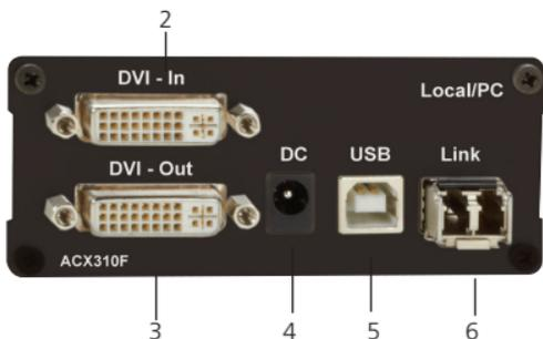
Figure 2-2. ACX310F-T transmitter's back panel.
