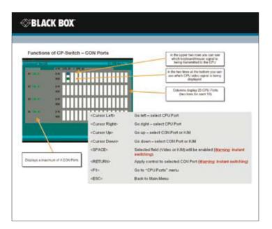
Matrix (cross point) mode: set video and K/M on different ports
