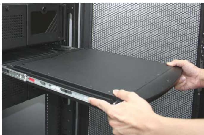
Figure 8. Pushing the white arrow button.
