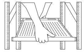
2. Slide the shelf to the depth of the rails and install the four plastic rivets as shown in the diagrams below.
