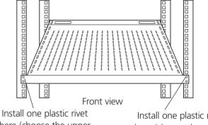
here (choose the upper hole from the two holes on the shelf that are lined up with the rail)
