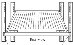
Install one plastic rivet here (choose the bottom hole from the two holes on the shelf that are lined up with the rail) Install one plastic rivet here (choose the bottom hole from the two holes on the shelf that are lined up with the rail)
