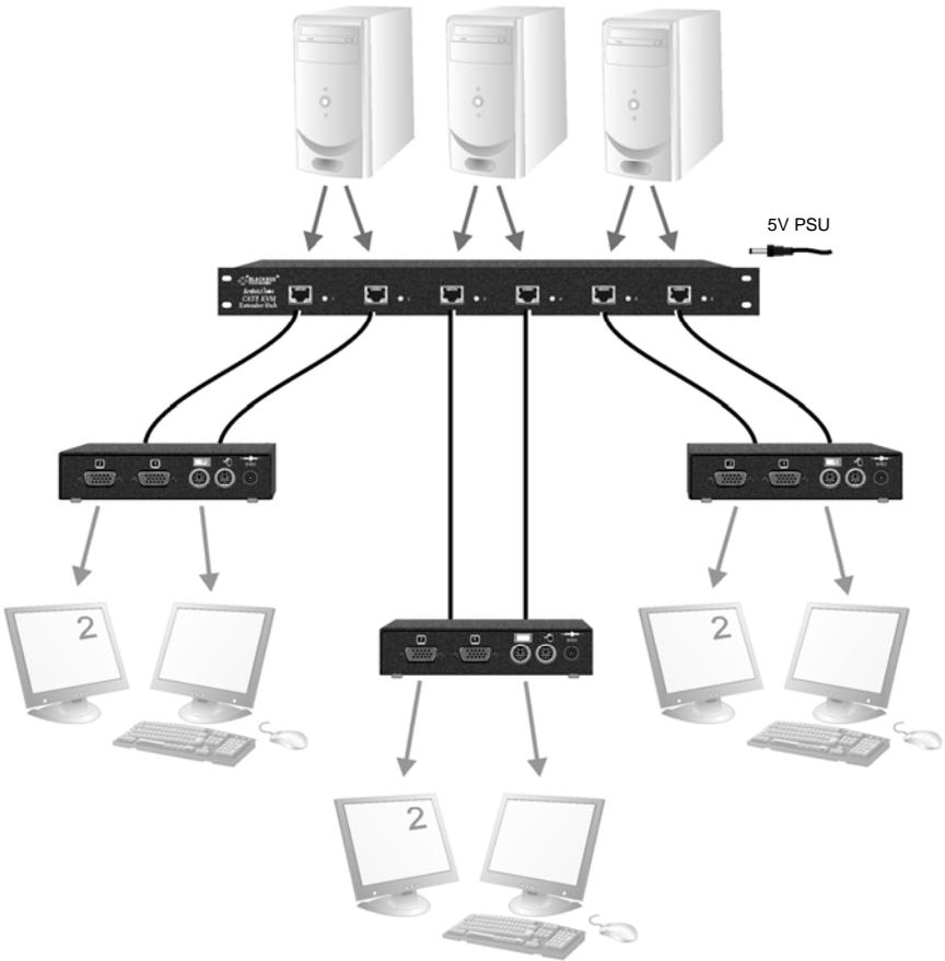
**Figure 6** ACU1006RA rack used with ACUMR02A Remote Units to extend dual video
