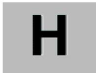
**Loss of Sharpness:** Loss of high frequency (HF) signals causes blurring and lack of detail. To correct this requires adjustment of *HF equalization*.
