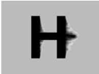
**Smearing:** black smearing at the right-hand edge of large horizontal objects such as title bars and characters. To correct this smearing requires adjustment of *LF equalization*.
