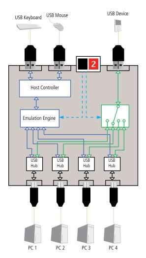
The inside view of a True Emulation USB switch. The emulated section of the switch is shown in blue and handles only the keyboard and mouse. This section relies heavily on the emulation engine, a custom circuit that is closely allied with each of the USB hubs. These ensure that all connections to the computers remain active.
